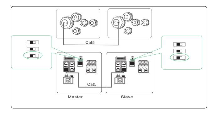
The connection diagram of three battery systems could be read below.
