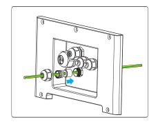
8. Strip the grounding cable and make the length ( L on the right drawing ) stripped 2-3 mm longer than the tube of the conductor (E on the right drawing).
