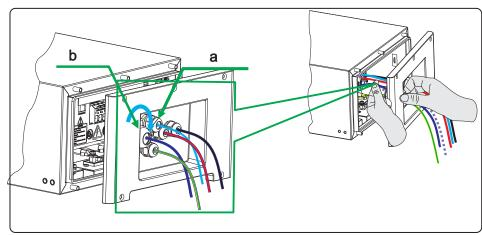
3. Fix the Operating Panel. To do this, insert the screws (M4x14) through the holes on them, using a Phillips screwdriver (PD2) and tighten it (torque: 2 Nm).
