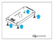
2. Put the installed base and feet along the wall, and keep the distance of 12~19 mm between the wall and the base.
